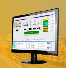
control the aggregates, admixtures, cement types, and water sources used in their production of any ordered concrete mix. The unique flexibility of the eBatch system allows the plant operator to synchronize and optimize concrete production schedules even when batch mixes change. While a batch mix is coming to the end of its processing, eBatch loads the new formula and begins preparing raw materials for the new batch process, which improves production time of the plant.
